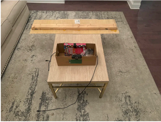
Fig. 1: Overall experimental setup, showing Walabot RF sensor, camera, and reference geometry.
